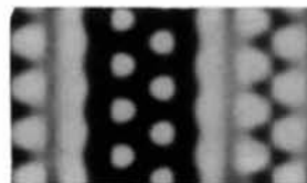
Fig. 11. The a -axis calculated image of a triple chain where all the T_1 , T_2 , T_7 and T_8 sites are occupied by Co. The crystal thickness t = 4 nm.
